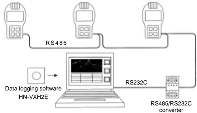
Note: Memory data can't be utilized because HN-VXH2E (RS485) is limited to the real-time measurement.
